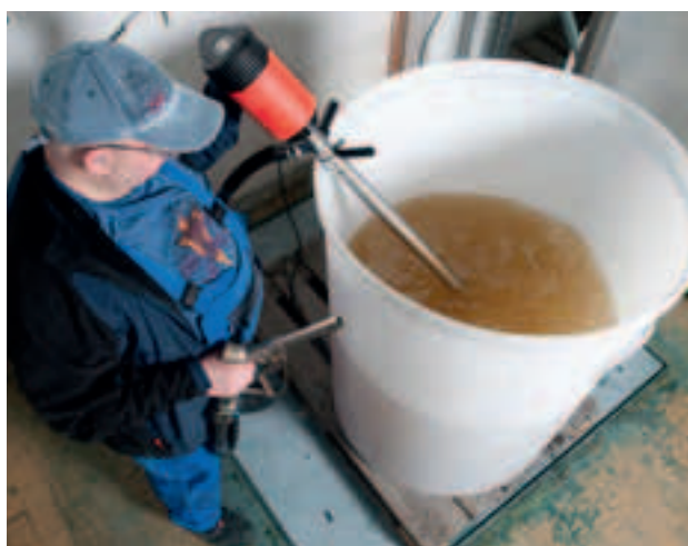
With the F 426 inhomogeneous media can be mixed before filling.
