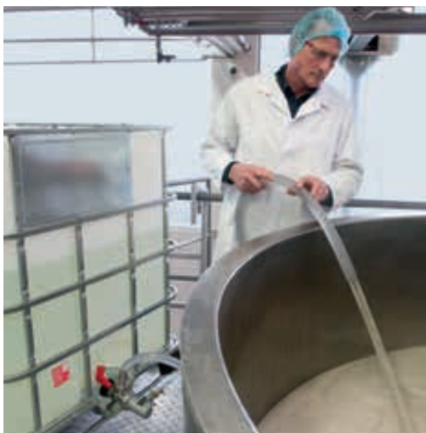
Pumping upward into a mixing container from the IBC outlet.
