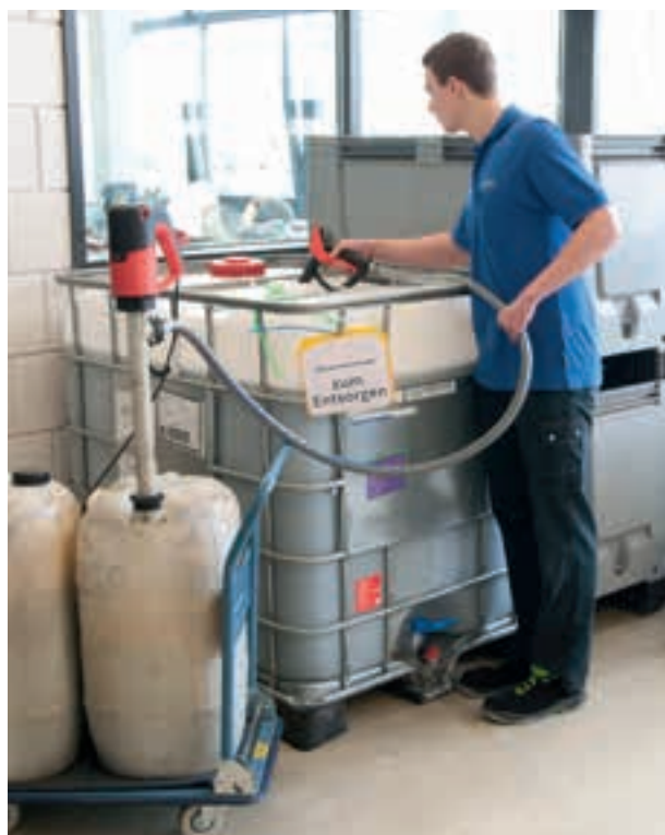
Disposal of mixed old chemicals (F 424 PP).
