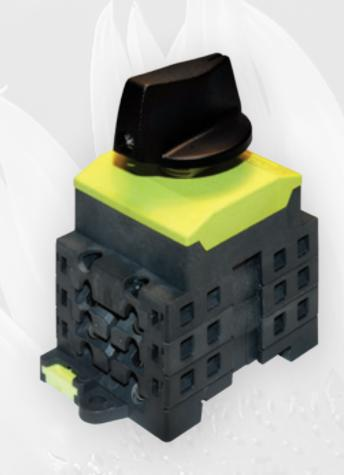
The operating principle of the Santon X-type is identical to the existing successful Santon DC switches which have been used throughout the world where DC switching is required as for example in the rail and shipbuilding industry. The prime characteristic for the Santon DC switch is its short switching time of approximately 3 ms, which reduces the arc forming to a minimum.
