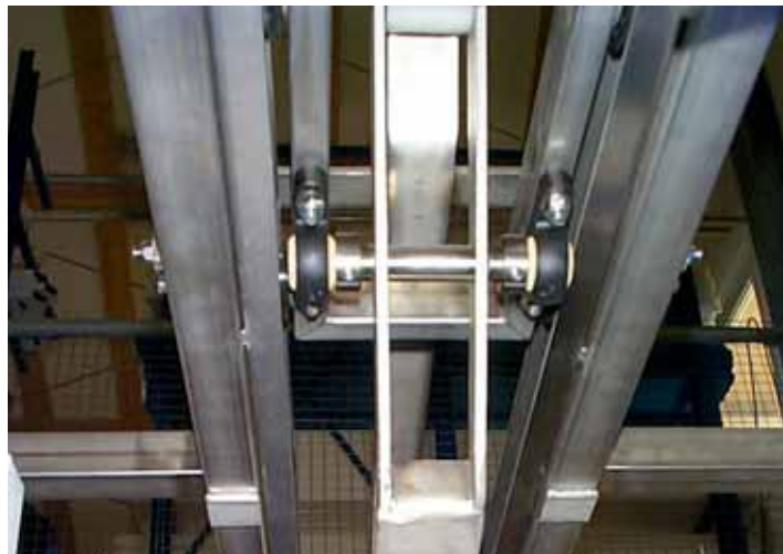
Picture 53.3: Application picture of igubal® pillow block bearings in the conveyor system
