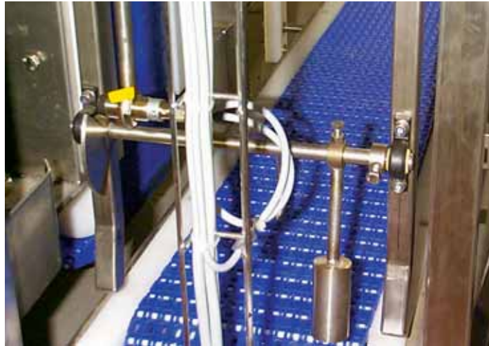
Picture 53.2: Application picture of igubal® pillow block bearings in the conveyor system
