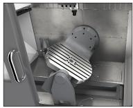
The UMC-750's integrated dual-axis trunnion table can position parts to nearly any angle for 5-sided (3+2) machining, or provide full simultaneous 5-axis motion for contouring and complex machining.
