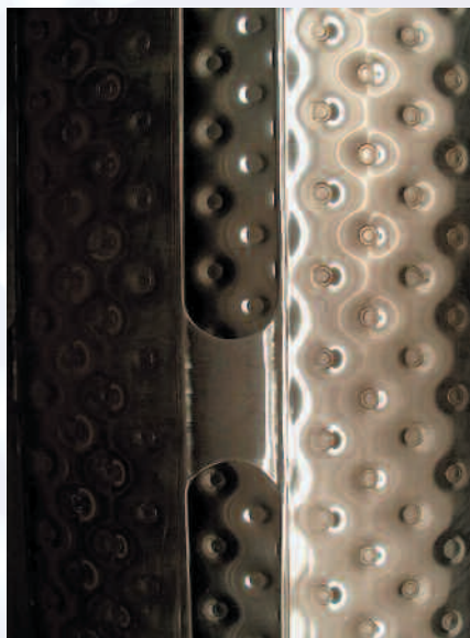
Condenser of short path evaporator in hygiene design
