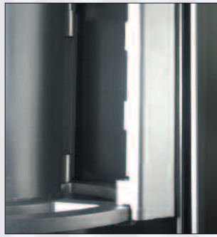
Rotor with hinged metal wiper blades
