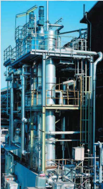
Two-stage thin film evaporation plant for resin concentration
