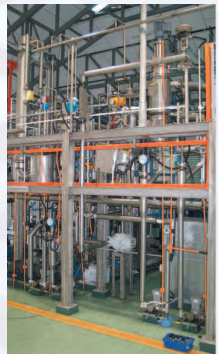
Pilot plant for methyl ester evaporation
