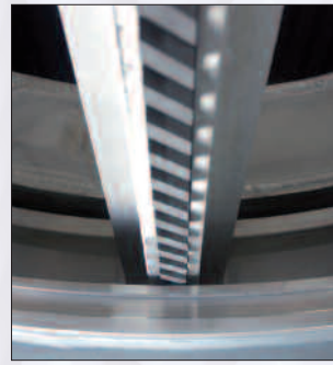
Rotor with radially moving PTFE or graphite wiper elements
