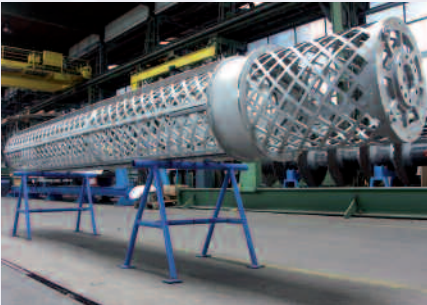
Rotor with radially moving PTFE wiper elements
