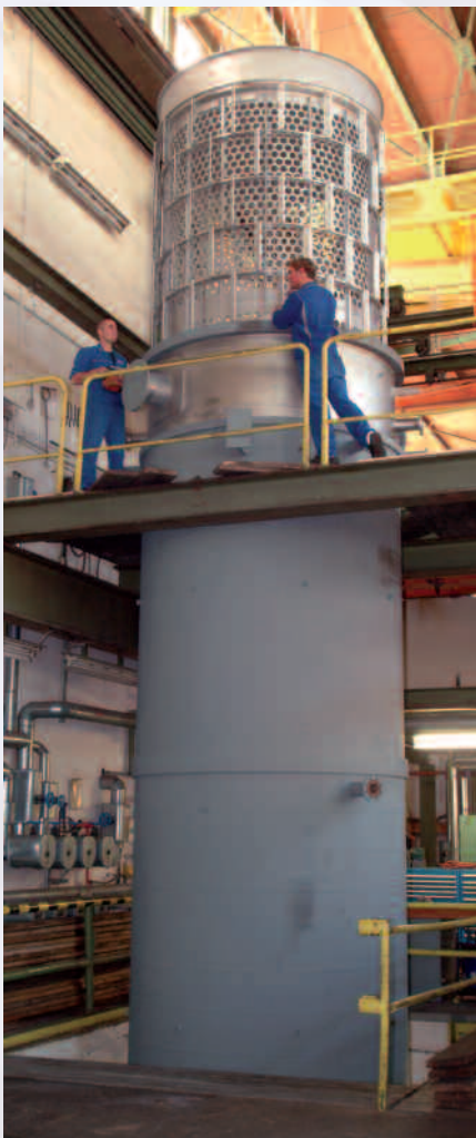
Thin film evaporator in our test facility
