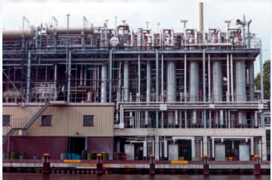
Multi-stage falling film evaporation plant for miscella distillation
