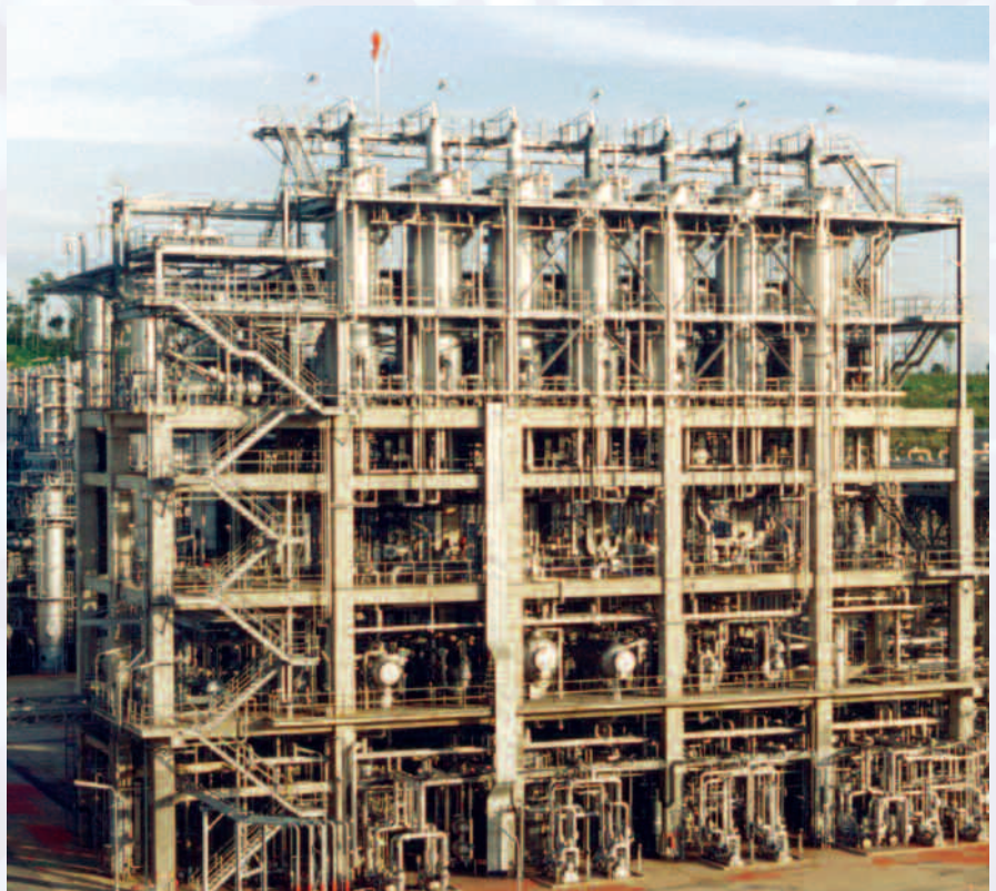
Largest multi-stage short path evaporation plant in the world for the production of soft and hard waxes
