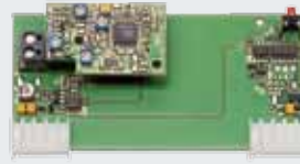
Receiver HER 1 (1-channel) with volt-free relay output in a separate housing without connecting lead or as a plug-in circuit board in the control cabinet
