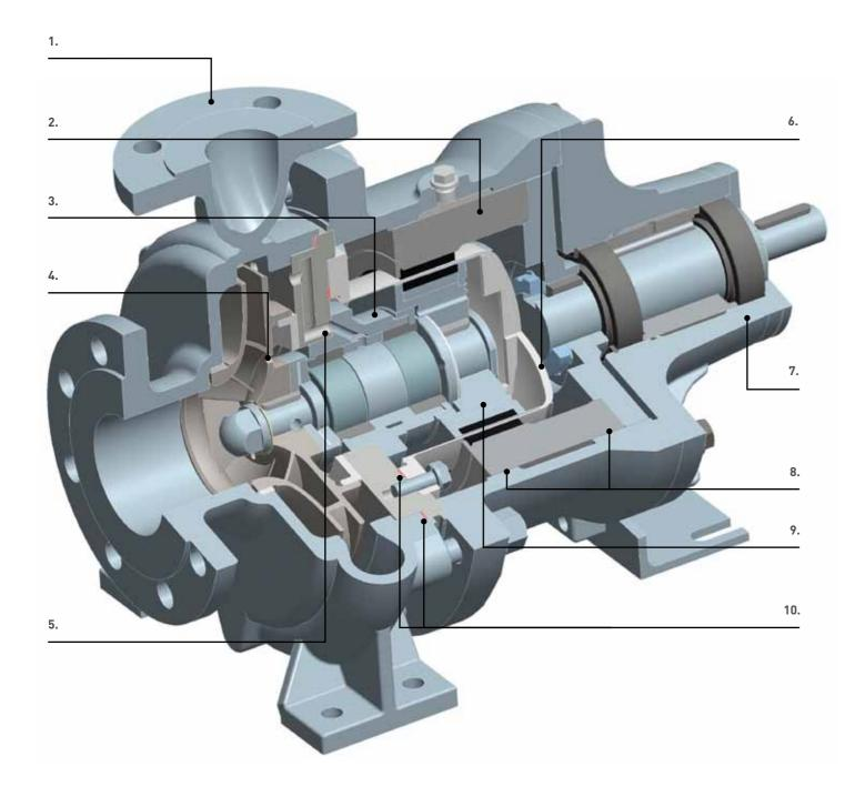
1. Pump casing PN 16 at 120 °C
