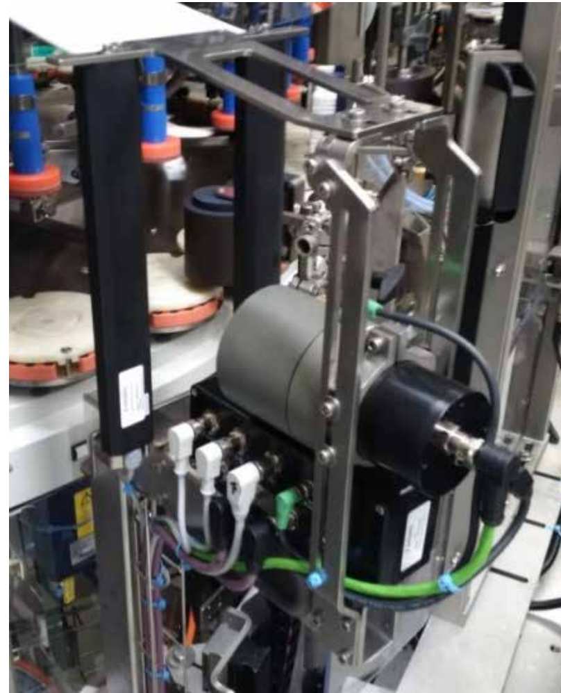
New: Efficient inspection with only one camera (picture: without enclosure)
