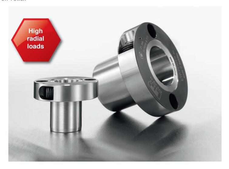
ETP-POWER is available as standard for shafts 15-40 mm. Runout  $\le 0,03$  mm. Number of mountings 200-500 (size dependent). ETP-POWER combines quick mounting with a high radial load capacity due to the specially developed pressure medium.
