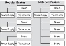
of each web or strand. This is most commonly attained by using a closedloop servo control system which controls current to a braking device through the use of dancer arms, follower arms and in-line tension transducers. The problem with such systems is that each web or strand must be individually controlled, increasing the cost and complicating the system with multiple sensors and power supplies.
