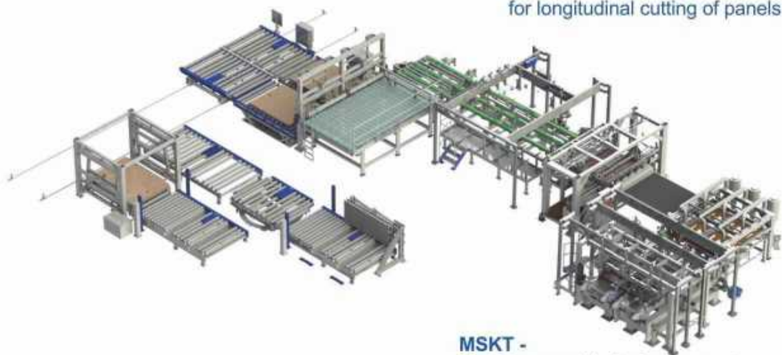
MSWT - Multirip saw with transport rollers for longitudinal cutting of panels
