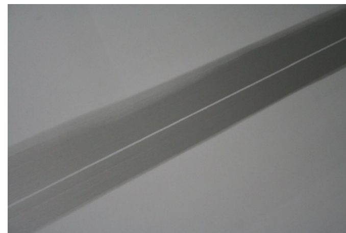
经酸洗处理，带轧制光泽，焊缝已磨去
