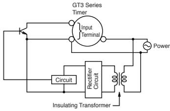
Connect the input signal terminals of the GT3A timers to Terminal No.2 only. Never apply voltage to other terminals; otherwise, the internal circuit may be damaged.
