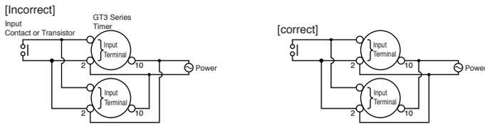
In a transistor circuit for controlling input signals, with its primary and secondary power circuits isolated, do not ground the secondary circuit.
