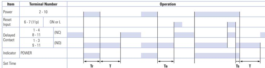
When power is applied, the NO contact closes. When power is removed, the timing period begins. When time has elapsed, the NO contact opens. Optional reset input will return contacts to original state before time elapses.
