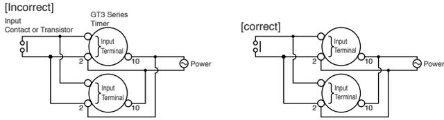
In a transistor circuit for controlling input signals, with its primary and secondary power circuits isolated, do not ground the secondary circuit.
