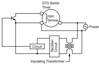
On the GT3F timers, connect the input signals to terminal No.1 and 4 only on the 8-pin type; connect the input signals to terminal No. 6 and 7 only on the 11-pin type. Never apply voltage to other terminals; otherwise, the internal circuit may be damaged.
