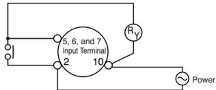
Input signal lines must be made as short as possible and installed away from power cables and power lines. Use shielded wires or a separate conduit for input wiring.
