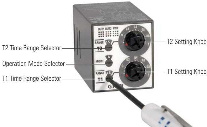
1. The switches should be securely turned using a flat screwdriver 4mm wide (maximum). Note that incorrect setting may cause malfunction. The switches, which do not turn infinitely, should not be turned beyond their limits.
