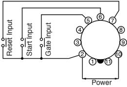
For transistor input, use transistors with the following specifications; VCE = 40V, VCES = 1V or less, IC = 50 mA or more, and ICBO = 50μA or less. The resistance should be less than 1kΩ when the transistor is on. When the output transistor switches on, a signal is input to the timer.
