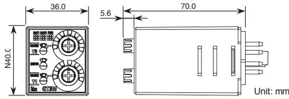
NOTE: GT3W series are UL Listed when used in combination with following IDEC's sockets:
