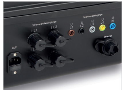
Fig.: Measurement connection for current transformer and voltage; auxiliary voltage and ethernet connection
