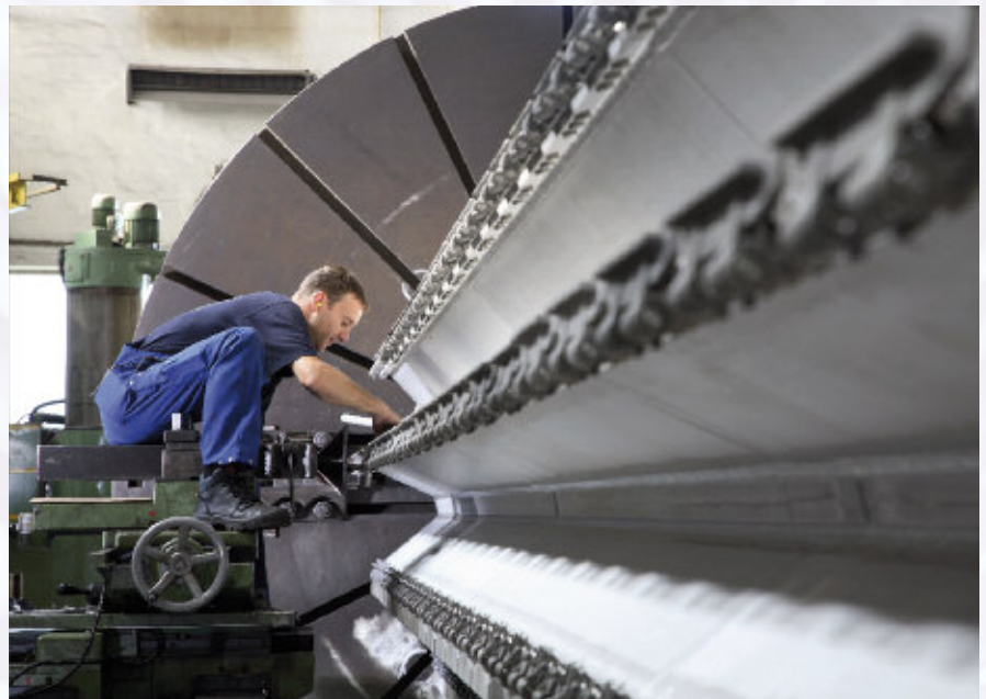
Manufacturing of CP rotor
