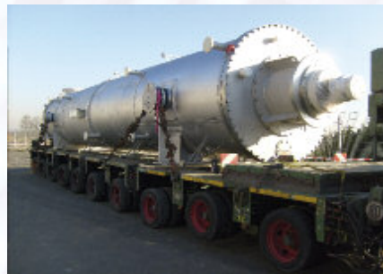
Transport of thin film dryer for food industry
