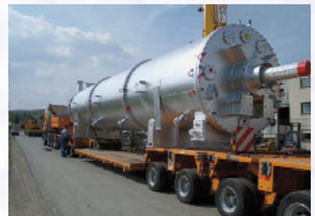
Transport of sludge dryer
