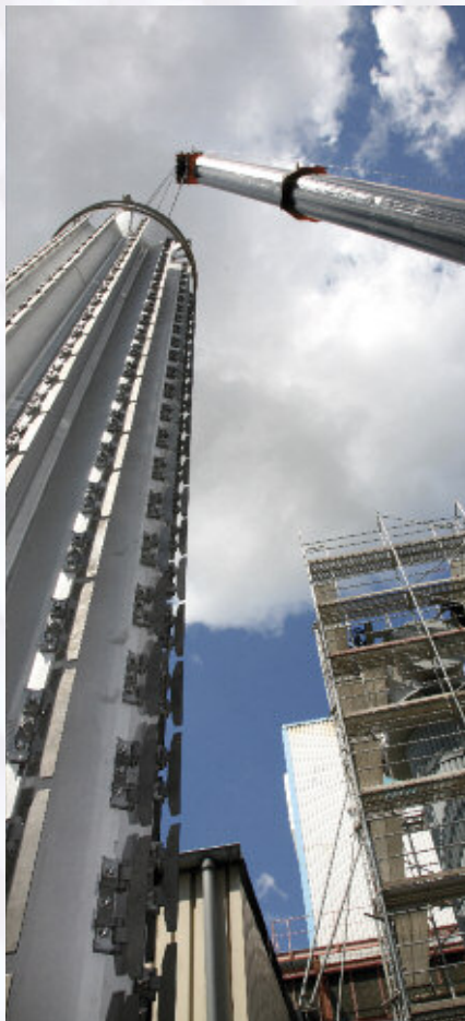
CP dryer in outdoor test stand
