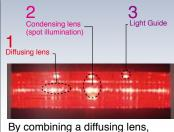
which diffuses the light broadly, with a condensing lens, a super bright area is created enabling high visibility. Also, the illumination through the light guide enhances the visibility when the SignaLight is viewed from below.
