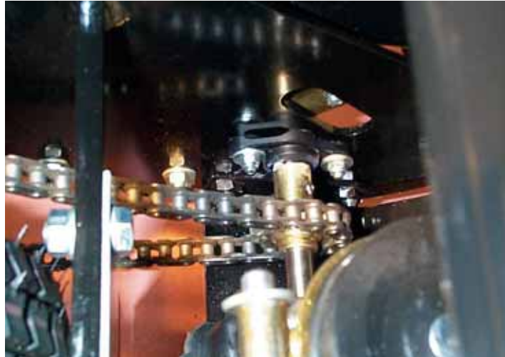
Picture 54.4: igubal® flange bearing in the drive shaft of the outdoor cleaning machine
