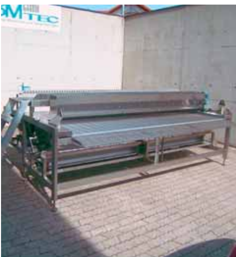
Picture 54.5: Leaching system for bakery products (for details see picture 54.6)
