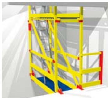
Lateral side protection to the right of the shaft door opening
