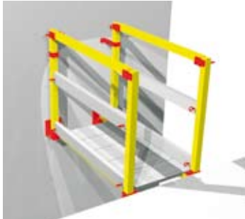
Service platform with three-part lateral protection
