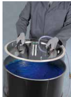
Assembly follower plate with process seal.*
