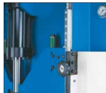
One or two 28 tons pressure cylinder
