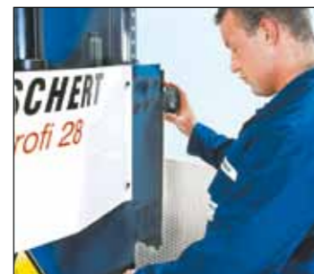
Stroke length adjustable under pressure
