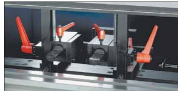
Side and height adjustable depth stops
