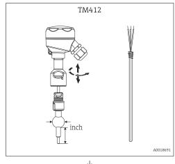
TMx**0**x characterizes the device that uses basic technology, with features such as a fixed, non-replaceable insert, application in non-hazardous areas, standard extension neck, low-cost unit
