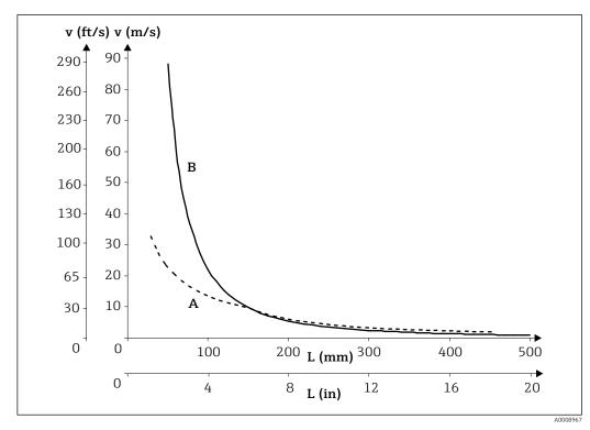
■ 6 Permitted flow velocities, protection tube diameter 9 mm (0.35 in)
