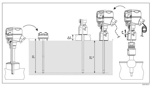
**■** 2 *Minimum insertion lengths for sensor calibration*
