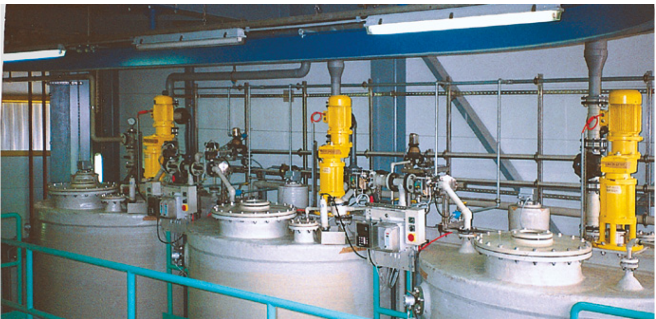
System to alkalyze influent stream with limestone.
