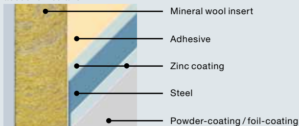
Mineral wool insert (on request) for better thermal insulation
