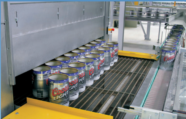
Internal bake oven curing party drums
