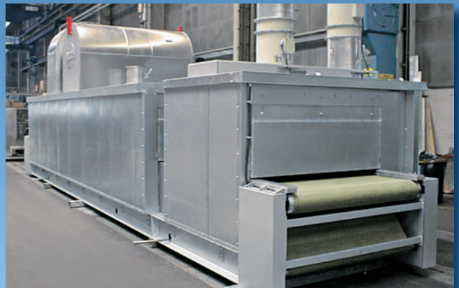
Single zone belt oven curing twist-off cap compound using a synthetic conveyor belt
