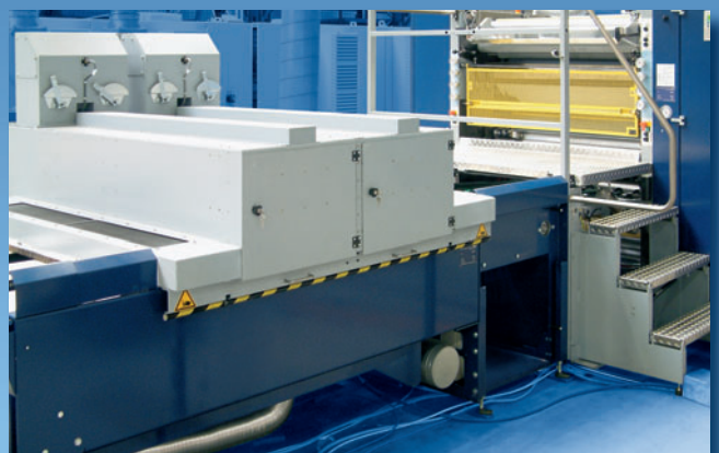
UV end dryer behind a MAILÄNDER printing machine
