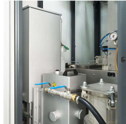
De-oiler & fine filter integrated in the housing
