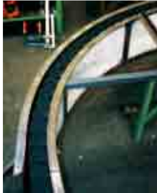
Guide troughs for rotary motion applications
