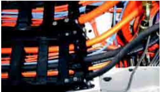
Chainfix strain relief in mounting bracket in practice - used here for cables and hoses
