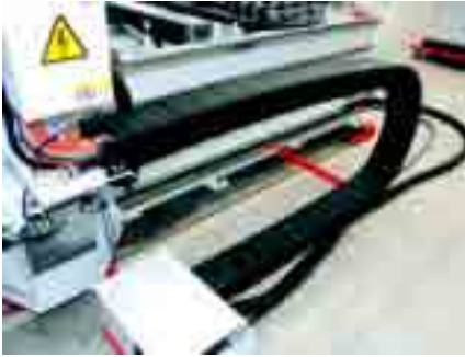
Pre-harnessed E-Tube for machining centers. E-Tube protect cables against dirt and chips
