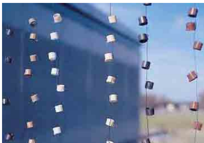
Picture 1.18: iglidur® plain bearing in UV test
