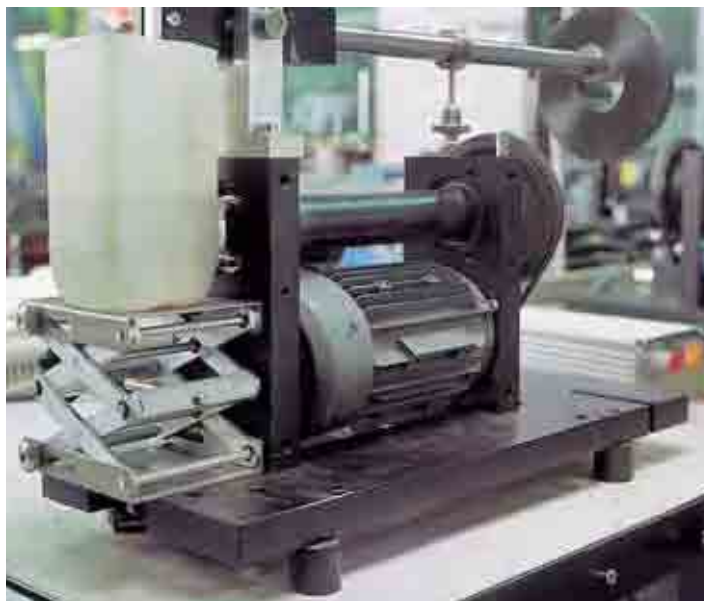
Picture 1.17: Rotational test centre for underwater and/or chemicals
