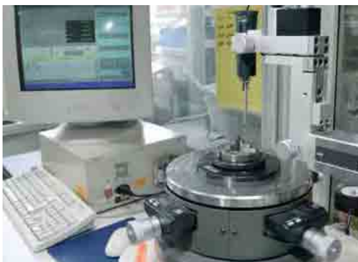
Picture 1.19: Measurement of the inner diameter of a pressfit plain bearing
