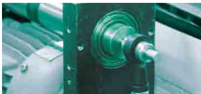
Picture 1.8: Determining the maximum surface speeds of an igubal® rod end bearing
