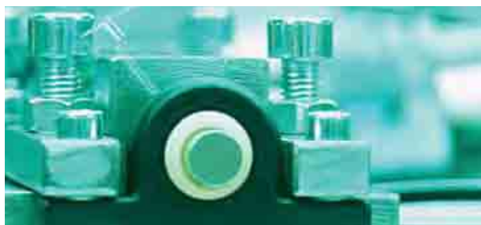
Picture 1.7: Experiments on wear and coefficient of friction with of an igubal® pillow block bearing
