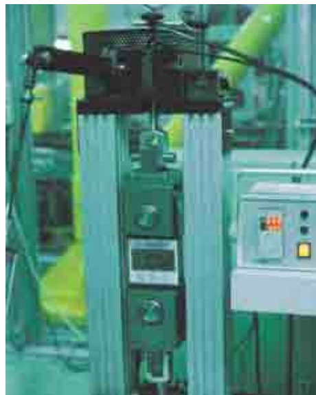
Picture 1.13: Test centre for high loads up to 150 MPa and temperatures up to 250°C, oscillating
