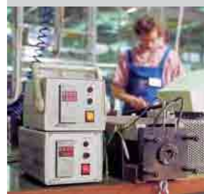
Picture 1.14: Wear test centre with temperature monitoring
