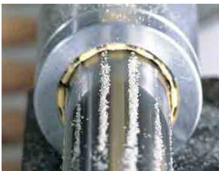
Picture 1.15: High wear resistance: plain bearing in contact with sand
