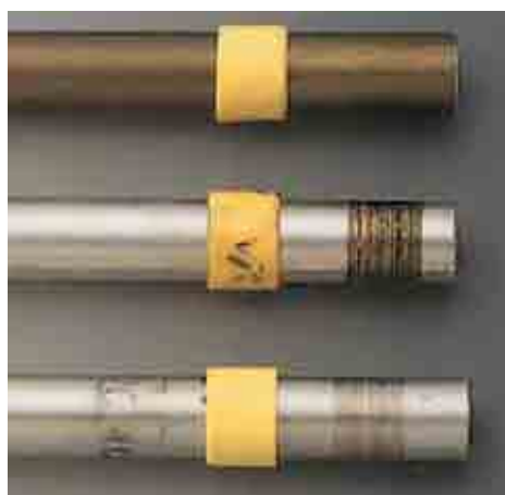
Picture 1.16: Wear experiments with aluminum shafts
