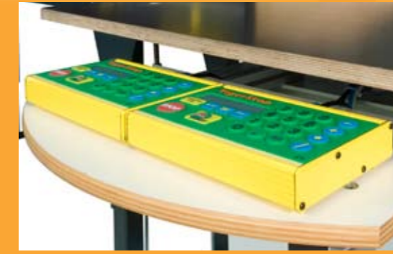
Automatic angle adjustment with Tigerstop Servo drive
