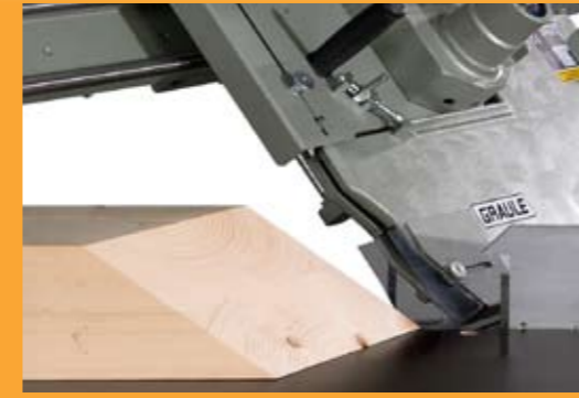
Maximum cross-sections up to 200 x 420 mm Precision 0,05 degrees
