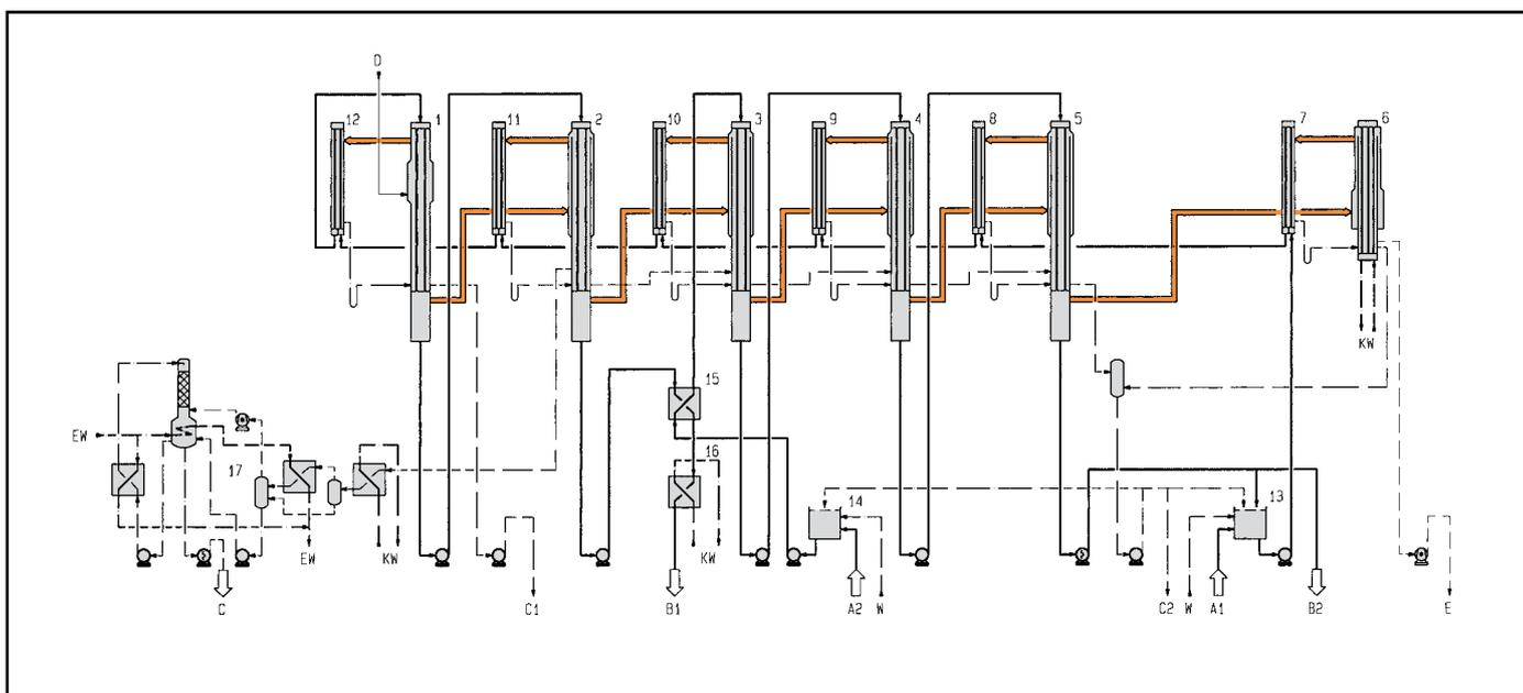
5-effect falling film evaporation plant, directly heated, with aroma recovery system (DIFFAR), concentrate cooling system and fining outlet, for apple juice
