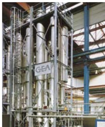
*4-effect falling film evaporation plant with aroma recovery system for apple juice, in compact design; evaporation rate: 8,000 kg/h*
