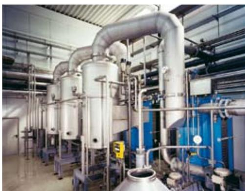
3-effect plate evaporation plant, directly heated; evaporation rate: 3,500 kg/h
