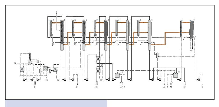
5-effect falling film evaporation plant, directly heated, with aroma recovery system (DIFFAR), concentrate cooling system and fining outlet, for apple juice
