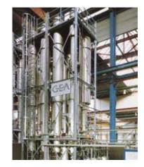
4-effect falling film evaporation plant with aroma recovery system for apple juice, in compact design; evaporation rate: 8,000 kg/h
