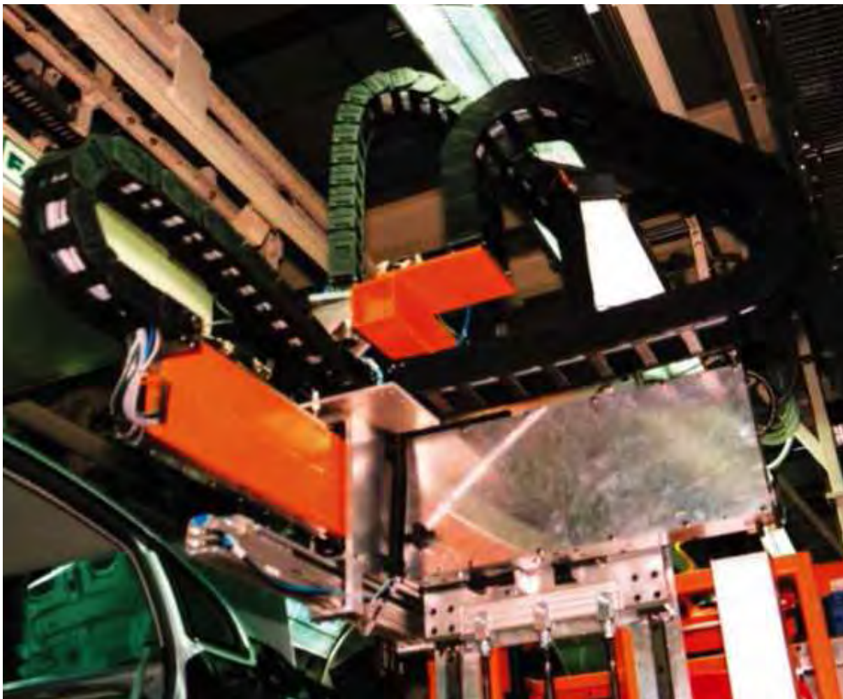
Three Energy Chain Systems® in several axes fitted with specially cables from igus®. E-Chain®: System E4/00 and System E4/0
