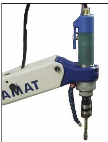
ROSCAMAT 400 E : Detail of the head with automatic tap lubrication system.
