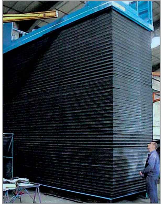
Bellows for elevating platform
