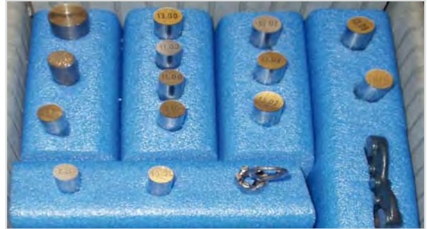
Material tolerance test on shearing components
