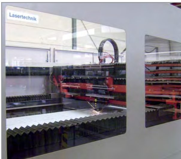
Bellows in operation
