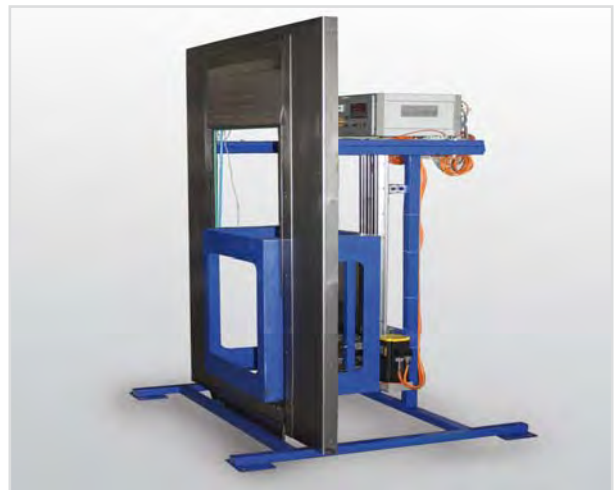
System test on the z axis with test on pneumatic components and guide rails
