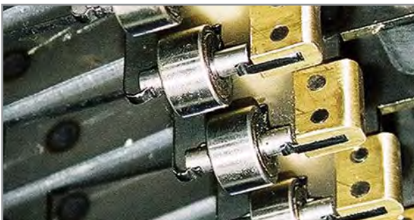
Supporting rollers with lateral brass guides
