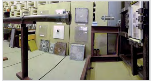
Impact test on safety screens under DIN EN 12415
