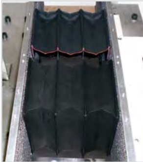
Material load test - flex fatigue strength at the corners of bellows
