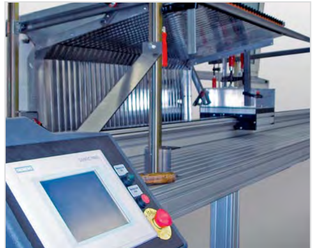
Traverse test on vector bellows with high accelerations up to 4 g
