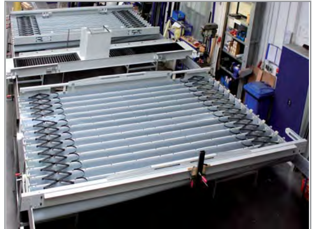
Roof cover with a length of more than nine meters, and a self-supporting width of more than five meters
