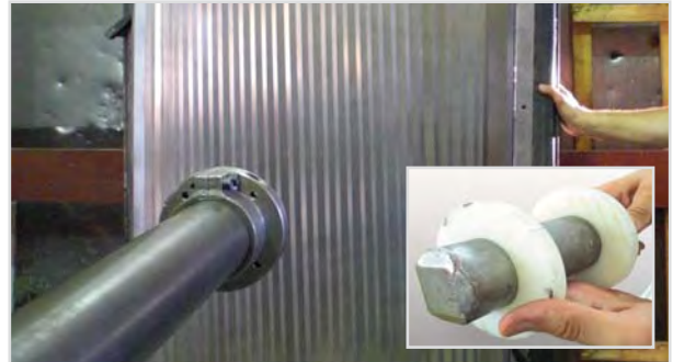
Impact test on covers under DIN EN 12417
