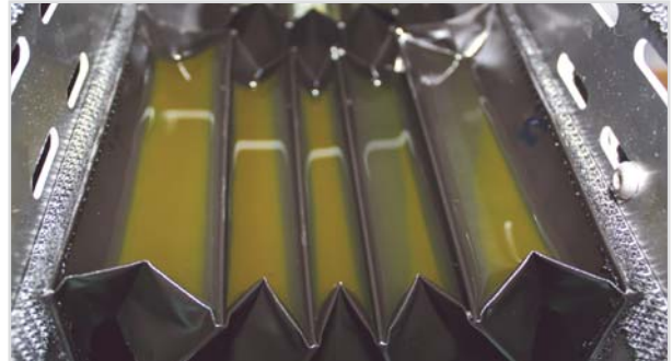
Static material load test - tightness test
