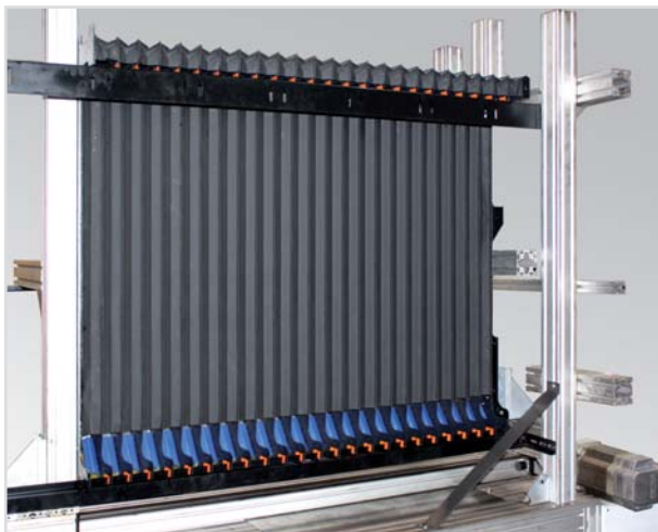
Traverse test on bellows service life and wear characteristics with up to three million cycles
