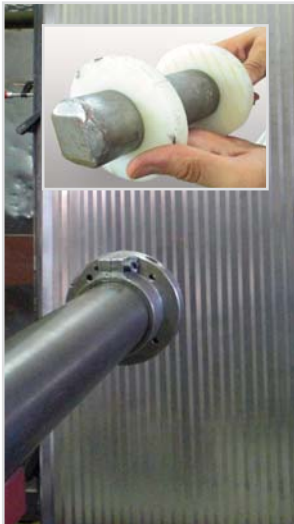
Impact test on covers under DIN EN 12417
