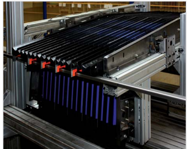
Traverse test on vector bellows with high accelerations up to 2 g
