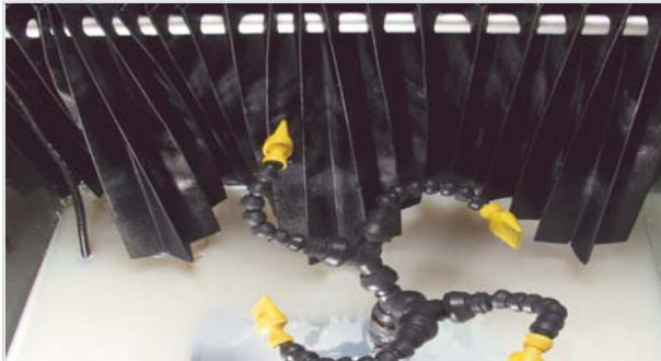
Material load test - coolant spray test, rotating nozzles
