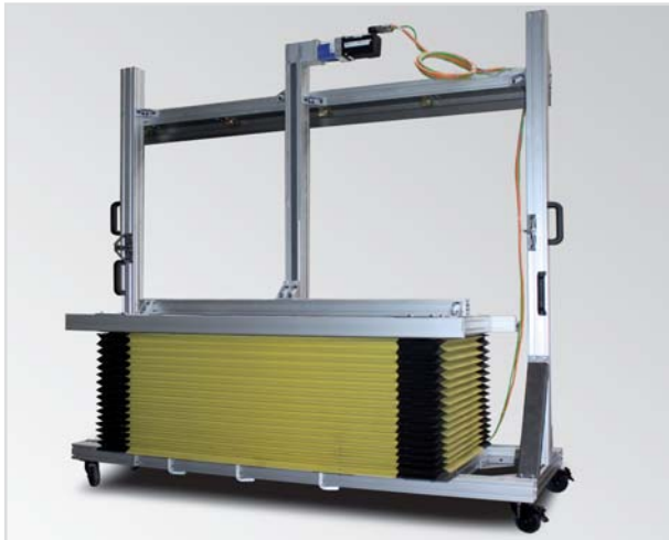
Endurance test on bellow service life and wear characteristics - bellow for lifting table
