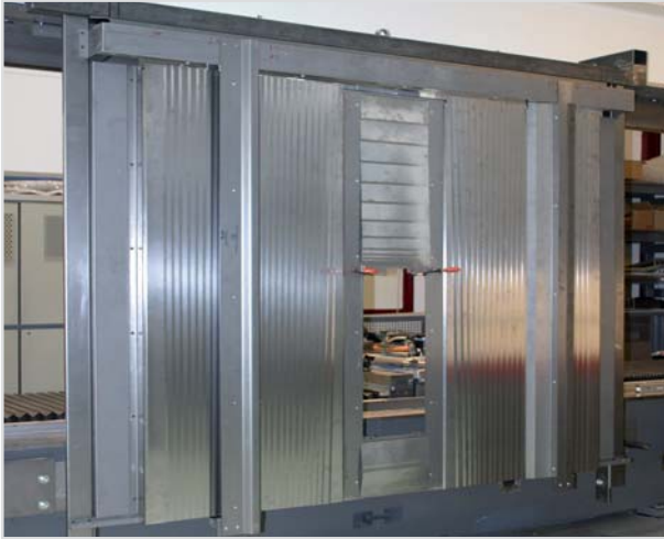
Function test for contact pressure and noise emissions from a complete rear wall on the PTW high speed test rig
