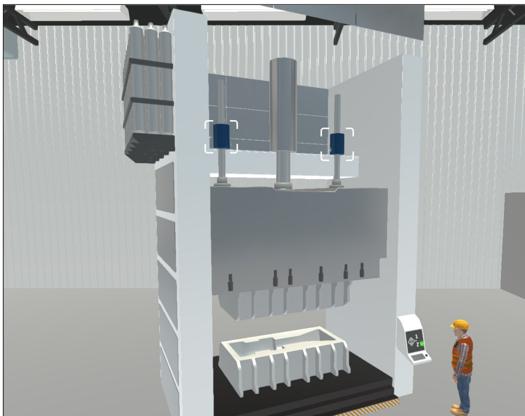
Fig. 1: Application example: schematic forming press with 2 x SITEMA Safety Catcher (interactive animation on www.sitema.com )
