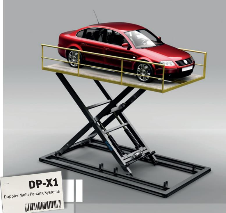
**DP-X1** is the perfect solution to connect parking levels and street without ramps. It is equipped with a sturdy hydraulic, scissors type, elevating mechanism, making it ideal for car dealerships and parking buildings. It requires a minimum pit depth while no shaft or guidance is necessary.
