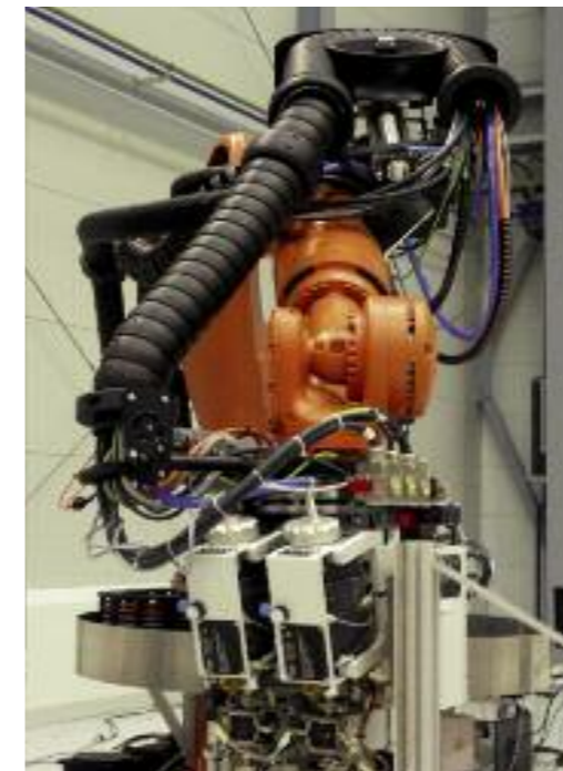
igus® chainflex® cables in application of a multi-dimensional moving energy chain triflex® R for 6-axis robots.
