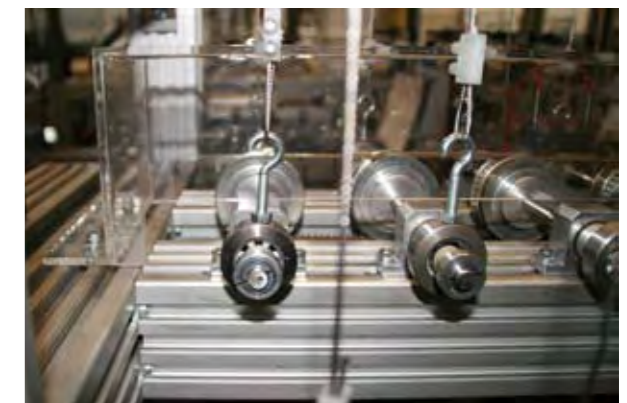
Ball Bearing test in igus® polymer lab
