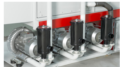
Lateral canal compressor (option) – optimised drying results
