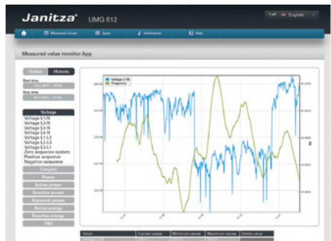
Fig.: Illustration of online and historical data via the homepage, above for example an APP - "Measured Value Monitor"
