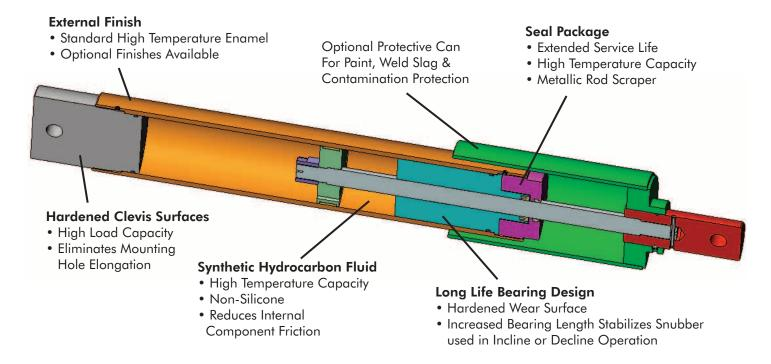
Enidine Tow Bar Snubbers reduce wear and downtime by absorbing high shock forces potentially transmitted into the moving carriage and its payload. These devices directly reduce maintenance costs associated with downtime and premature component wear.
