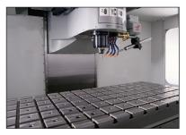
For versatile fixturing, VM Series machines feature a specially designed table that has T-slots in both X and Y directions, as well as precision dowel-pin bores and a pattern of drilled & tapped holes.
