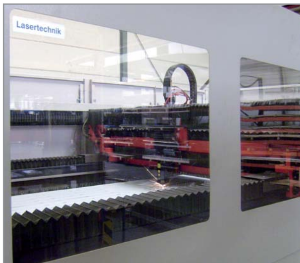
Bellows in operation
