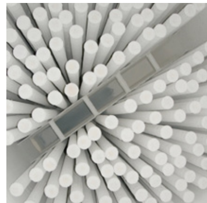
Hose filter, raw gas side
