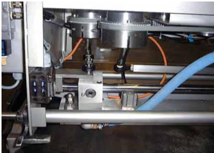
Picture 51.1: igubal® rod end bearings in a confectionery decorating machine
