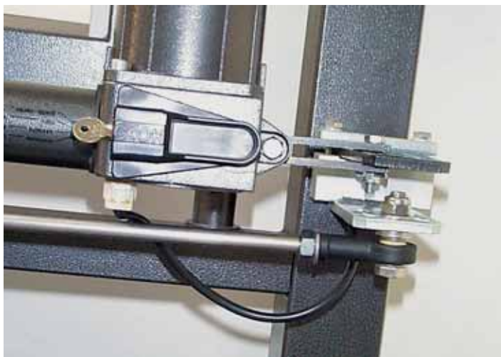
Picture 51.3: igubal® rod end bearings in the closing mechanism of an outdoor security gate
