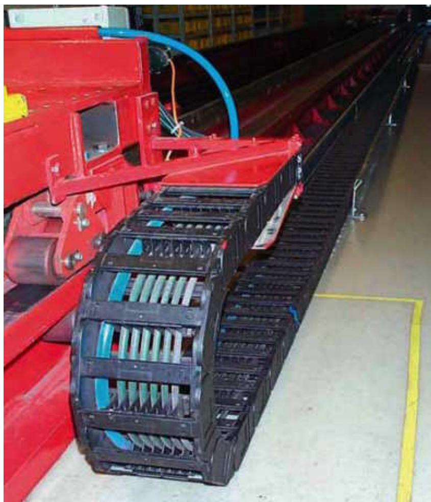
CF5/CF6 for shelf control units: long travel in the longitudinal axis. E-Chain®: Series E4/00 with igus® guide trough out of steel
