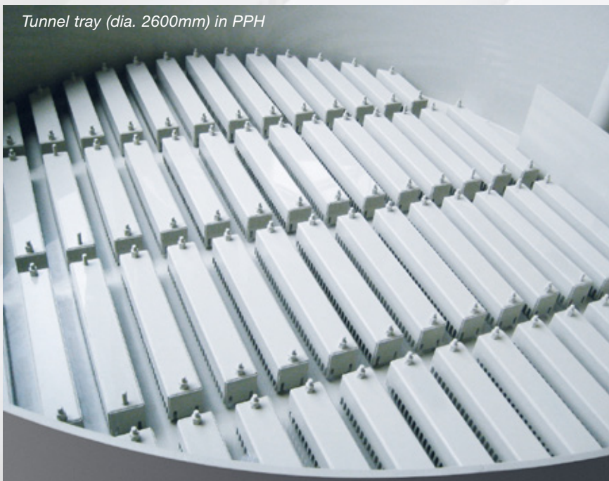
Installation of tunnel caps at a tunnel tray (dia. 2600mm)
