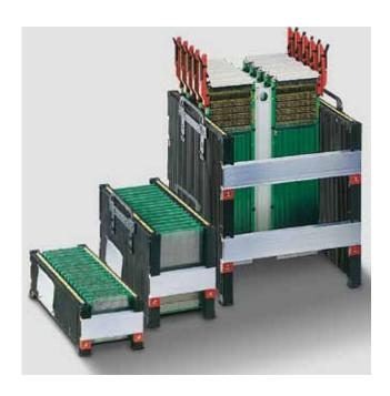
The cab PCB magazines can be filled when standing vertical or laying horizontal. The system is totally adjustable for width and can be assembled according to your individual requirements. For different size PCBs we offer PCB magazines with a height of 100, 180 and 300 mm.
