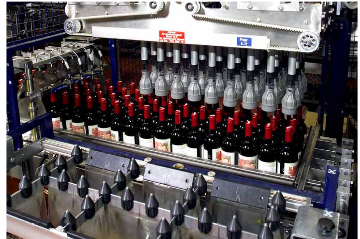
Spindle-adjustable gripper head for handling different container diameters
